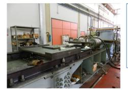
Driving of test bed for fatigue tests with servo-controlled oilhydraulic units (in cooperation with MASTEL)
